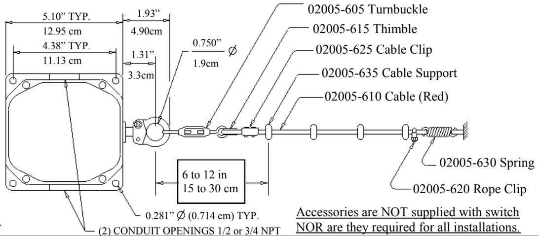
Note: Seal unused conduit opening(s) with approved plug(s).
